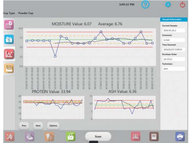
Configurable SPC view displays control charts for three constituents enabling immediate process control
